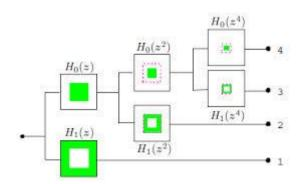
Figure 1: Three-stage non-subsampled pyramid decomposition.
