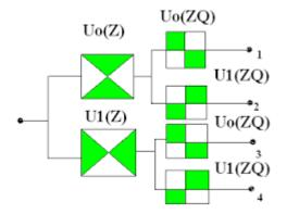
Figure 2: Four-channel non-subsampled directional filter bank.
